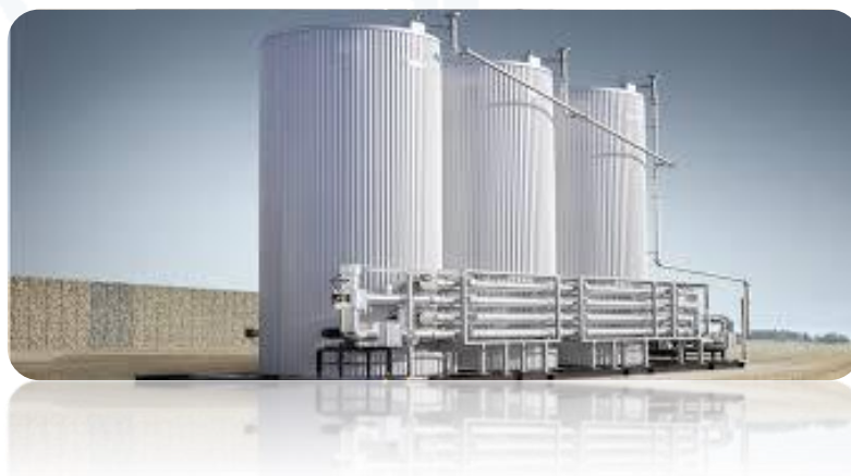
Figure 16. Storage silos of a bituminous emulsion.
