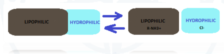
Figure 8. Schematization of the dissociation mechanism of a cationic emulsifier in water.
