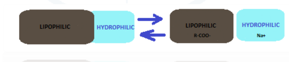
Figure 6. Schematization of the dissociation mechanism of an anionic emulsifier in water.
